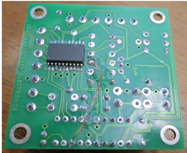
Remove R4 and install wire from r4 to pin 8 on IC1
