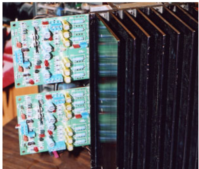
Power amp modules bolted to the heat sink.
