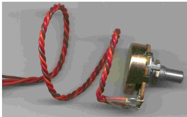
Fig 12. Potentiometer cable assembly for level and damping control.
