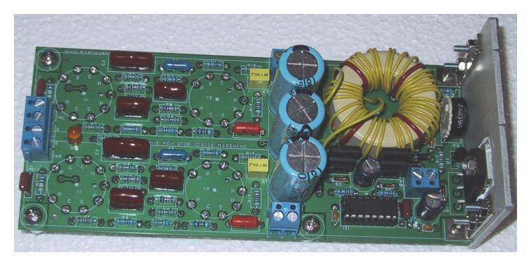
Components are installed in the usual way. Tube sockets on bottom (solder side) of the board . Install IC1 using 16-pin DIP socket. Fasten the brackets to the circuit boad using 3/16 M/F standoffs. Attach heatsink w.  $4 \#4/40 \times 1/2$ " screws. Use mica insulator w. thermal compound on both sides with transistor Q1. fasten w. #4 screw.
