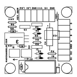
Remove R4 and install wire from r4 to pin 8 on IC1
